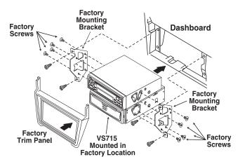
Figure 11. In-dash ISO mounting of the VS715.
